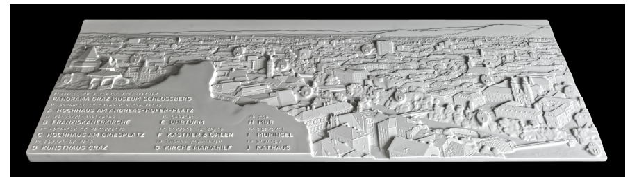
The finished 1260x450mm 2 large and 32mm high relief was CNC machined from DuPont Corian™, a material that is weather resistant, pleasant to the touch, does not heat up excessively in direct sunshine and can be machined to a high level of detail, a tremendous advantage over currently existing 3D printing processes. It was produced at the Department of Three-Dimensional Design and Model Making, Institute of Art and Design, Vienna University of Technology, especially by Florian Rist.
